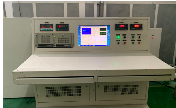
风量测试数据采集系统 Fan performance test data acquisition system
