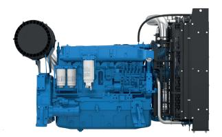
Bore x Stroke (mm) 126 x 130 Displacement (L) 9.72 N° of Cylinders 6 Cylinders Arrangement In line Open Chamber / Lean Burn Fuel System Governor (Gov.) EĊU Aspiration (Asp.) Turbocharged & air-to-air cooled
